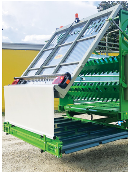
LATERAL ROLLER DISCHARGE WITH HYDRAULIC RETRACTABLE SIDE CONVEYOR
