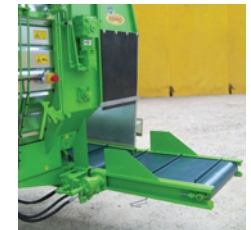
Conveyor belt extension
