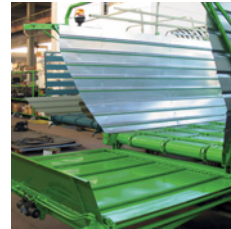
LATERAL UNLOADING CONVEYOR Door open
