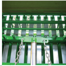
Self-loading elevator width: 1400 - 8/9/10 eased discharging blade system. Setup 9 shredding blades
