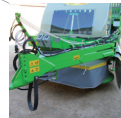
Double drawbar reinforced frame
