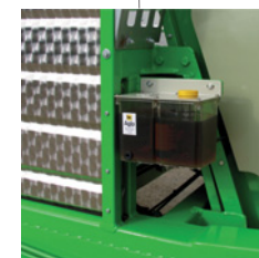
Automatic lubrication Self-loading elevator
