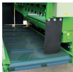
Conveyor belt width: 750 mm Side conveyor belt
