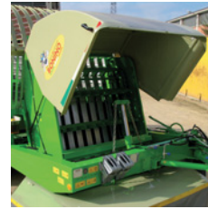
Fiberglass body with windows to access the grass elevator
