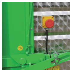
Automatic release emergency button on both sides
