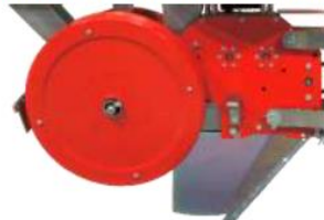
Standard iron ridging wheels Ø 500x80 mm
